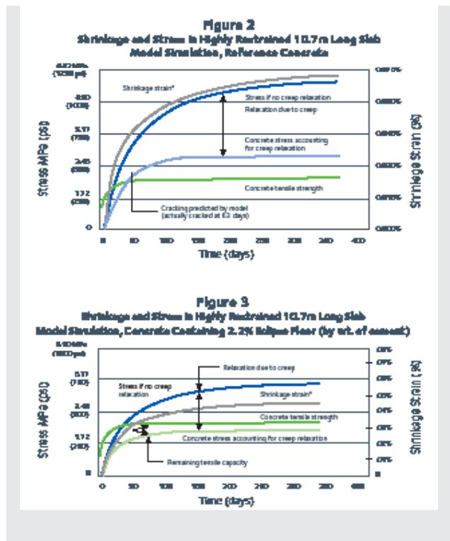
\* Shrinkage strain measured on unrestrained specimen. Actual large scale members were restrained causing stress to build up.
