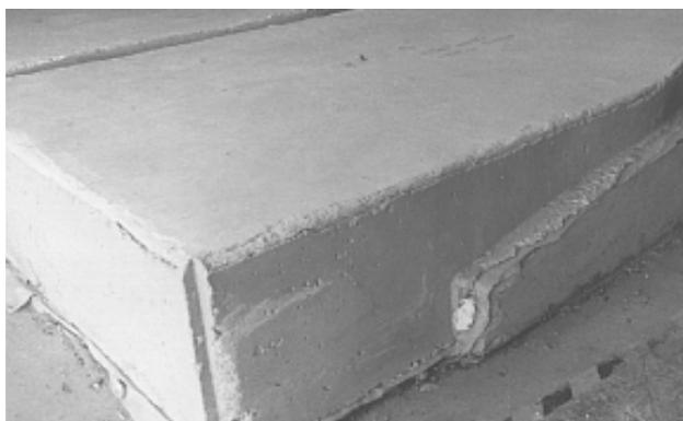
This close-up shows how test slabs were restrained by heavy steel-reinforced pre-conditioned bottom bases.
