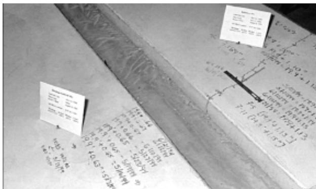
Side-by-side comparison (after 24 months) shows long-term performance of Eclipse Floor vs. the reference. The reference cracked in 2 months (at right). The slab containing Eclipse Floor is crack free (at left) after more than three years of continuous drying.
