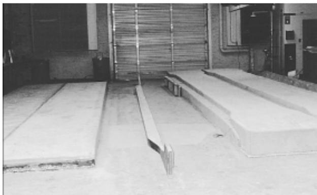
A converted 1920s ice cream factory in Cambridge, MA was the site for a full-scale restrained shrinkage test in a controlled environment. Two highly restrained slabs of identical composition, with the exception of Eclipse Floor, were placed and monitored for over 36 months.
