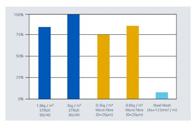
Note: The addition of STRUX 90/40 fibres, to control plastic shrinkage cracking, does not negate the need for appropriate and efficient curing techniques.
