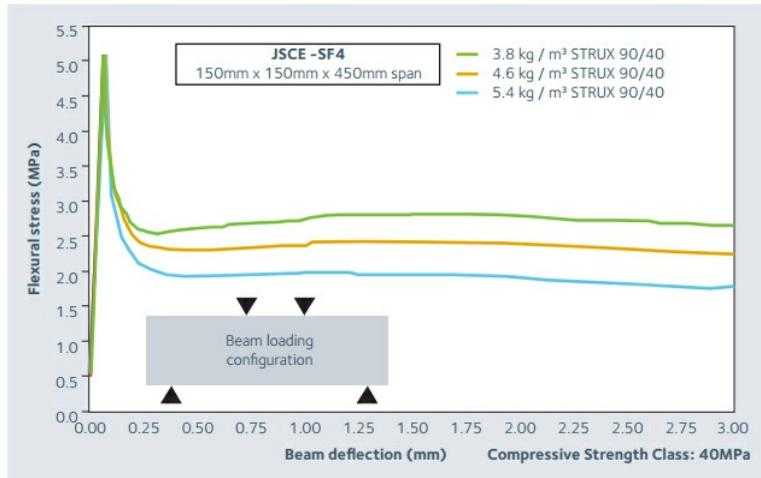
Note: These curves are based on averages of several beam tests. The toughness performance will depend on the concrete mix design used.
